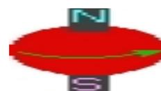
2. In the presence of an external magnetic field ( $B_0$ ), two spin states exist,  $+1/2$  and  $-1/2$ . The magnetic moment of the lower energy  $+1/2$  state is aligned with the external field, but that of the higher energy  $-1/2$  spin state is opposed to the external field. Note that the arrow representing the external field points North.
